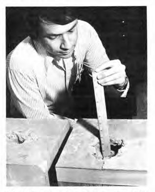
HOLES punched in solid concrete blocks in the laboratory by the drilling head average five inches in diameter, about three inches deep. Robert Silva (5724) displays a couple of the test blocks.
